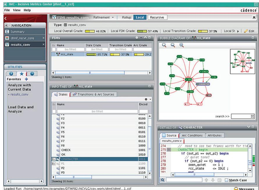
Figure 4: The Xcelium simulator provides the Cadence IMC for concurrent dynamic analysis views. Shown here: Context-aware activity for finite state machine analysis.
