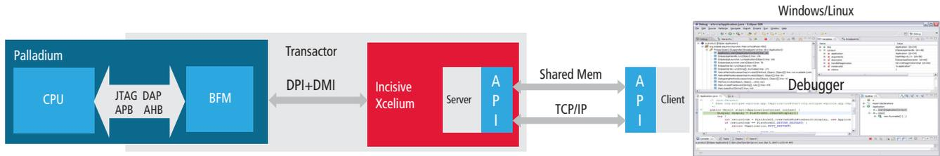
Figure 2: Block diagram overview of virtual debug interface
