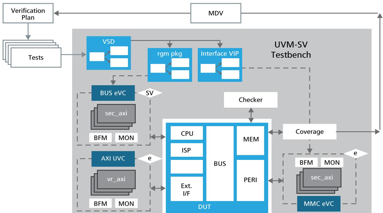
Figure 2: SoC verification environment
