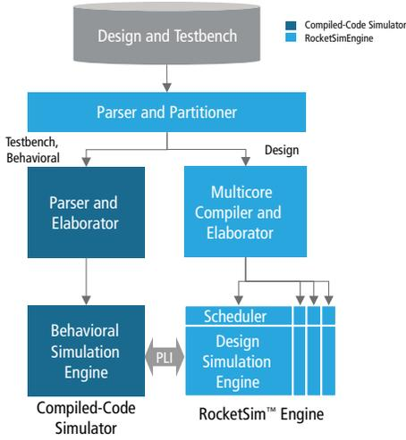
Figure 2: Integration of RocketSim engine and compiled code simulation
