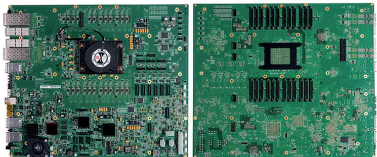
Figure 1: Protium S1 Single-FPGA Board (front and back views)
