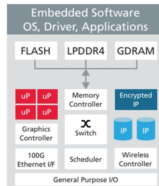
Figure 2: This example SoC design includes hardware and software.
