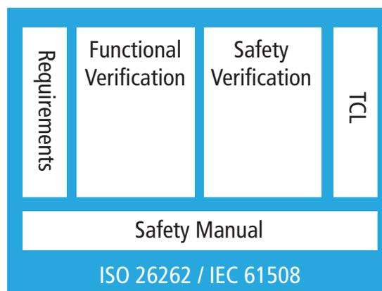
Figure 1: Elements of functional safety standards
