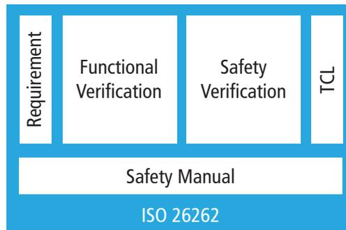
Figure 1: Elements of ISO 26262 from a verification perspective
