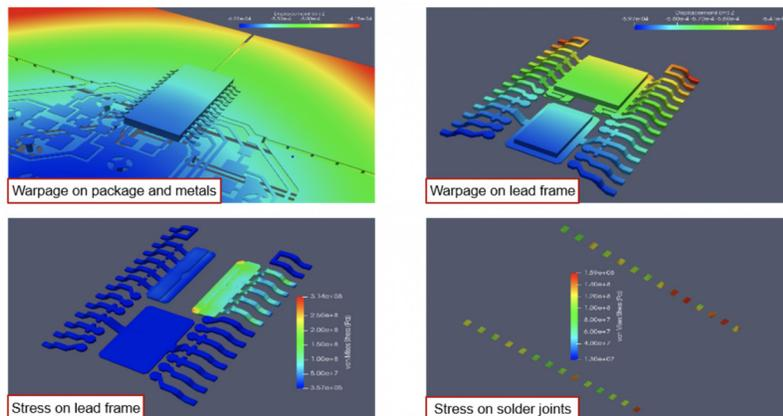
Figure 3: The Celsius Thermal Solver accounts for thermally induced stress.
