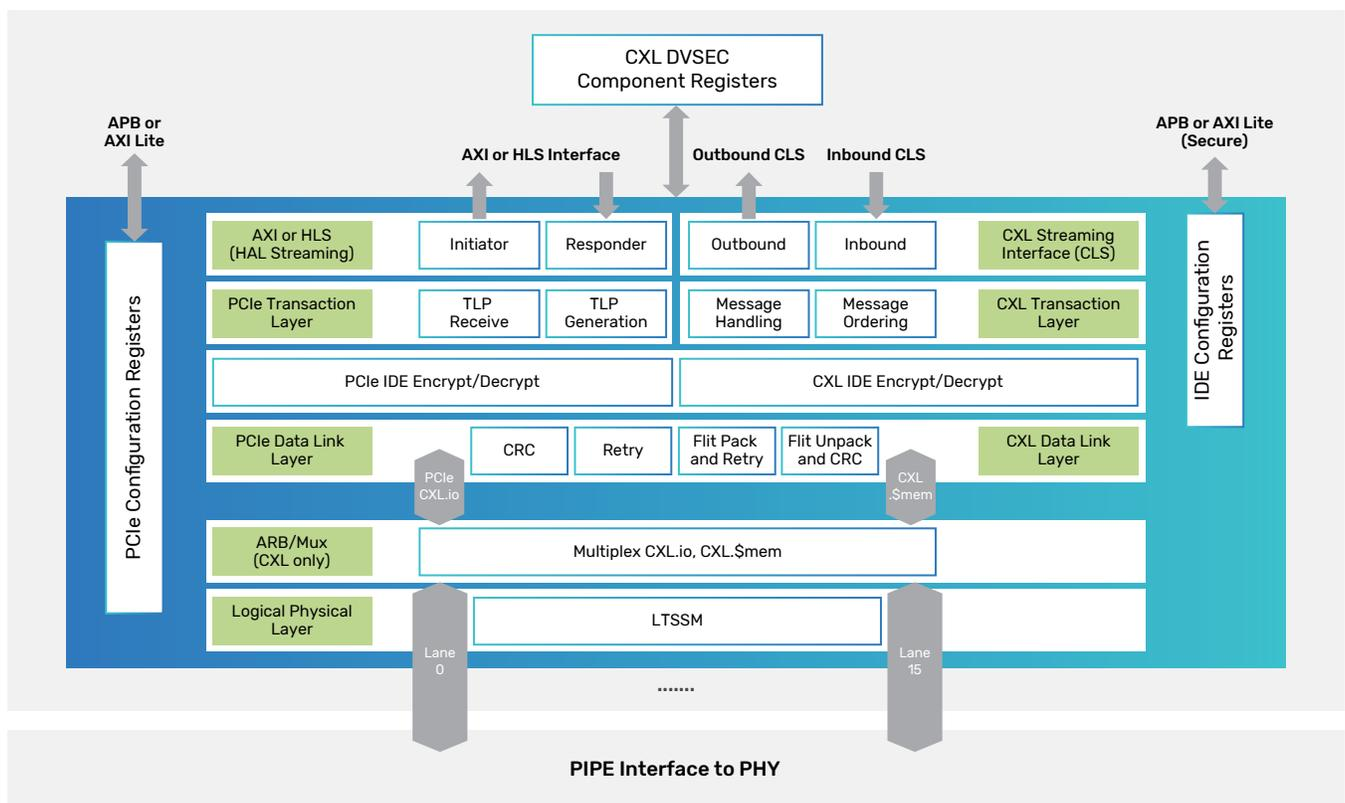
Figure 1: PCIe and CXL controller block diagram
