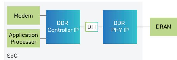
Figure 1: Example system-level block diagram
