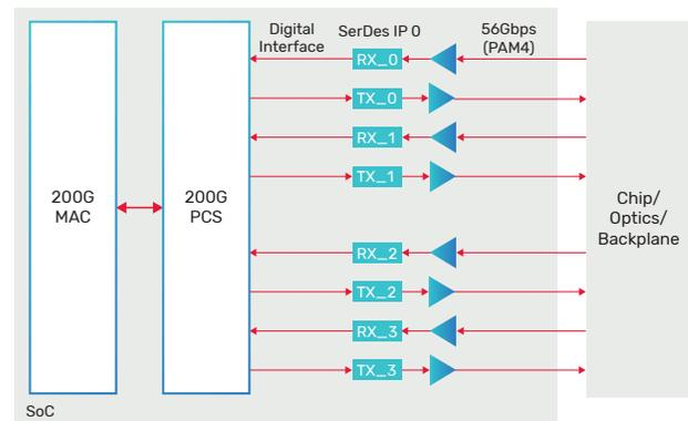
Figure 1: Example system-level block diagram
