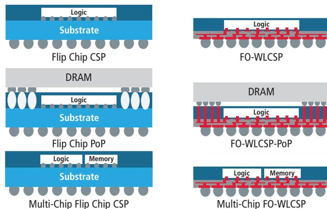
Figure 1: Examples of chip-scale-packaging compared with UT-FOWLCSP
