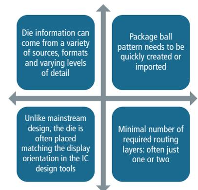
Figure 2: Some typical design challenges unique to UT-FOWLCSP implementations that must be managed by design tools and designers
