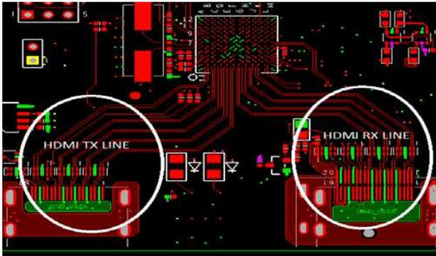
Figure 2: HDMI board layout: four lines for TX and another four for RX
