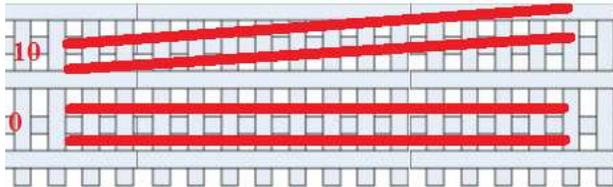
Figure 6: TX lines routed with 0° and 10° rotation on the PCB.
