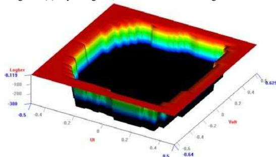
Figure 7(b): Bathtub curve plot, when 0° rotation routing on the board.
