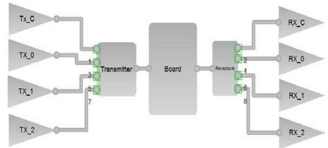
Figure 5: Test bench setup for HDMI channel simulation.
