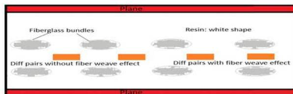
Figure 1: Cross-sectional profile of HDMI transmission line model with/without FWE.
