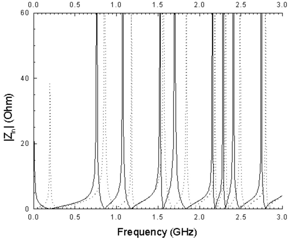
**Fig. 3 Input impedance of parallel metal planes. Solid line: two metal planes shown in Fig. 2(a). Dot line: two metal planes with a shorting via shown in Fig. 2(b)**
