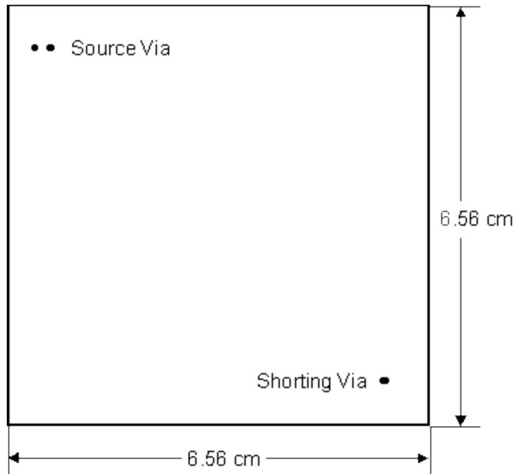
**Fig. 1 Top view of metal planes**
