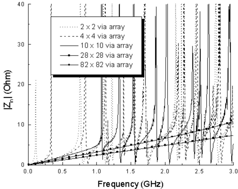
Fig. 7 Input impedances of different via array densities
