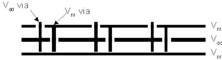
**Fig. 5 Metal planes of a package power supply system**
