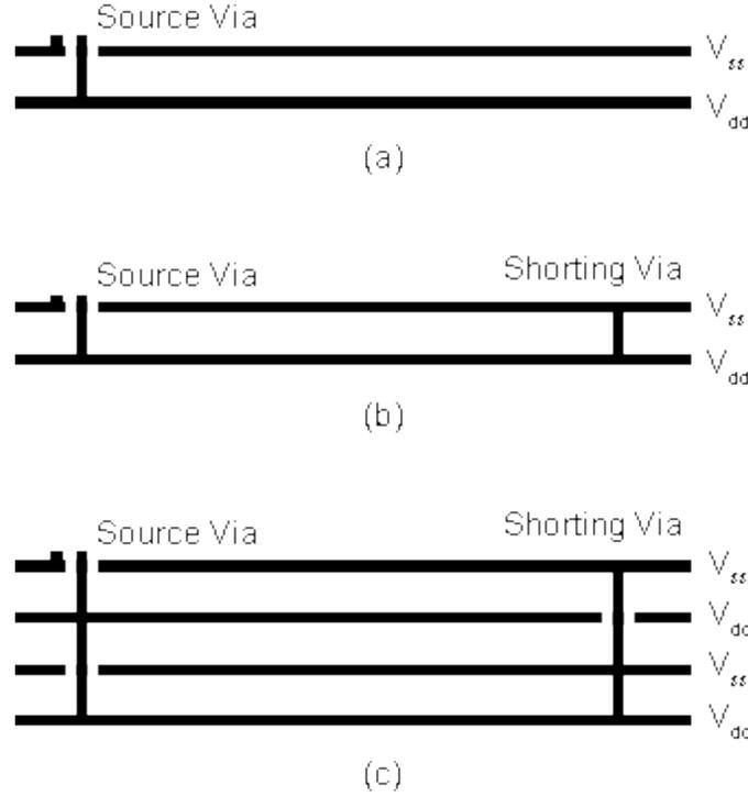
Fig. 2 Side view the metal plane configuration
