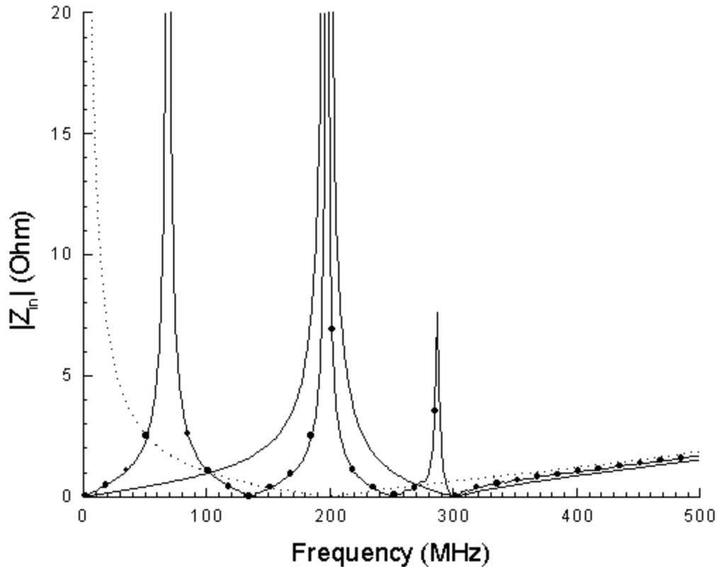
Fig. 4 Input impedances of multiple power and ground planes. Dot line: two metal planes shown in Fig. 2(a). Solid line: two metal planes with a shorting via shown in Fig. 2(b). Solid line with circles: four metal planes with shorting vias shown in Fig. 2 (c).
