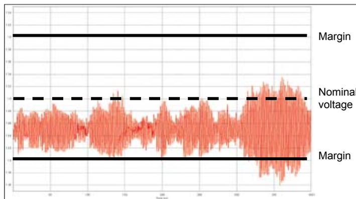
Figure 1: The migration from 130nm to 90nm has shrunk supply voltages to 1.2V and below, and increased currents supplied to devices through the PDS.
