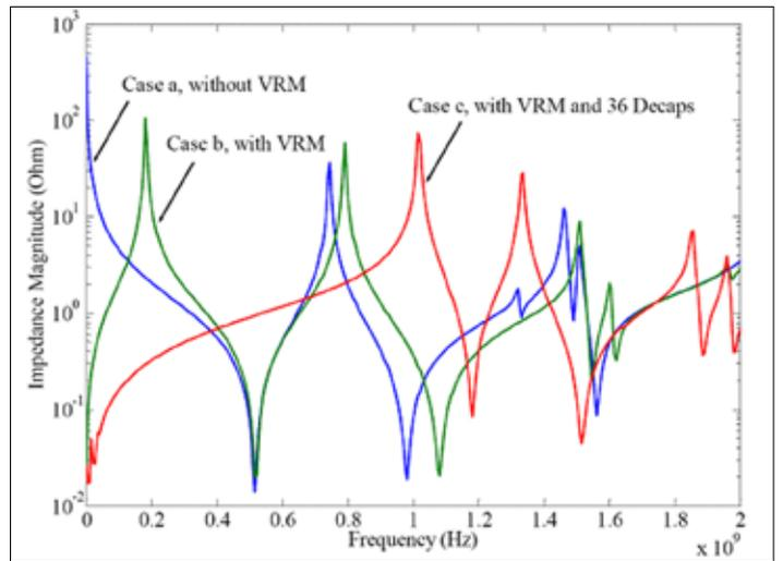
Figure 6: Shown is the input impedance of a PDS simulated by Sigrity PowerSI with three different scenarios.
