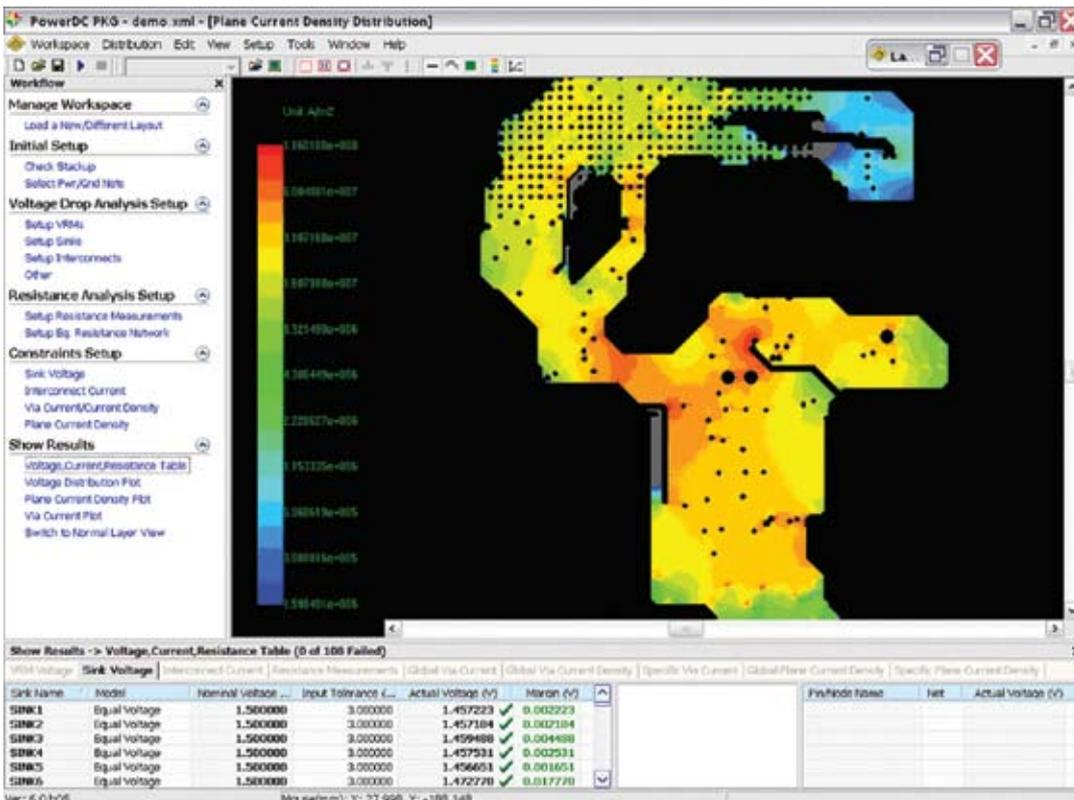
Figure 4: IR drop analyses can pinpoint critical voltage and current distribution in the PDS for a high-performance PCB.
