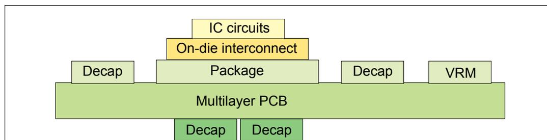
Figure 2: A PDS can be divided into three physical sections: silicon, IC package and PCB.
