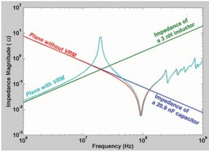
Figure 5: Figure shows the input impedance of a pair of planes as compared with the impedance of a pure capacitor and pure inductor.
