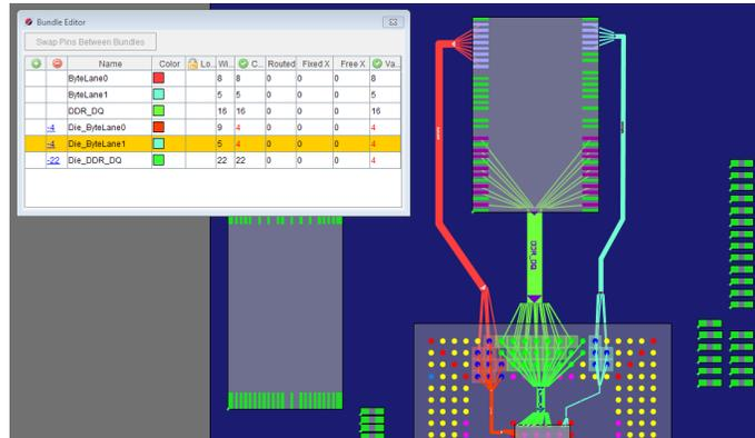
Figure 2: PCB-driven package and die assignment
