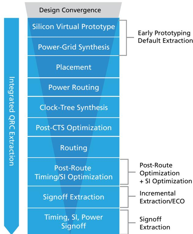
Figure 2: Quantus QRC Extraction Solution integrates with Encounter Digital Implementation System, together fostering better and faster design convergence.
