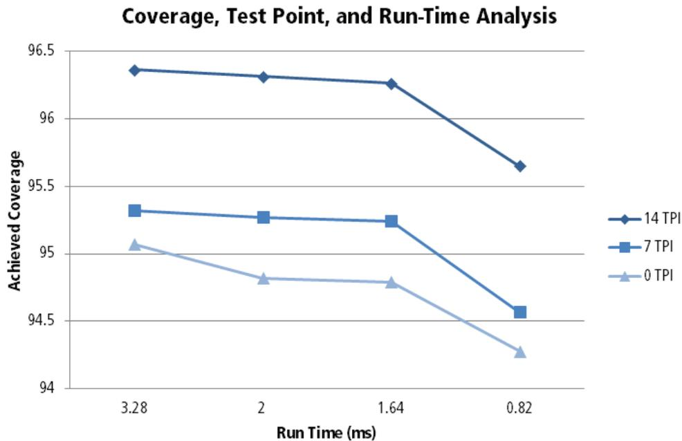
Figure 1: LBIST coverage at different run times and test points inserted
