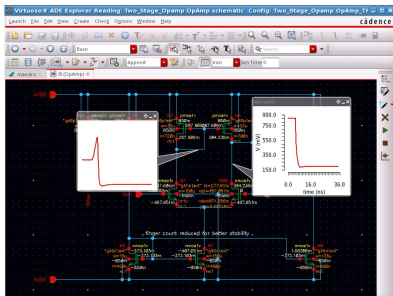
Figure 3: Schematic centric use-model showing waveform balloons
