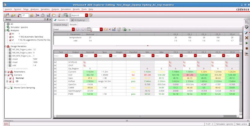
Figure 4: GUI-centric use-model showing corners and pass/fail status
