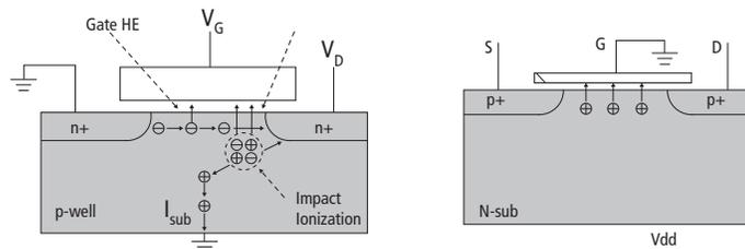
Figure 3: Hot carrier injection (HCI)
