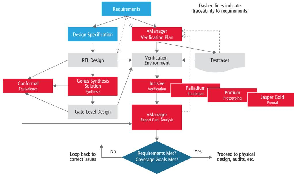
Figure 5: Tool flow diagram leveraging Cadence tools
