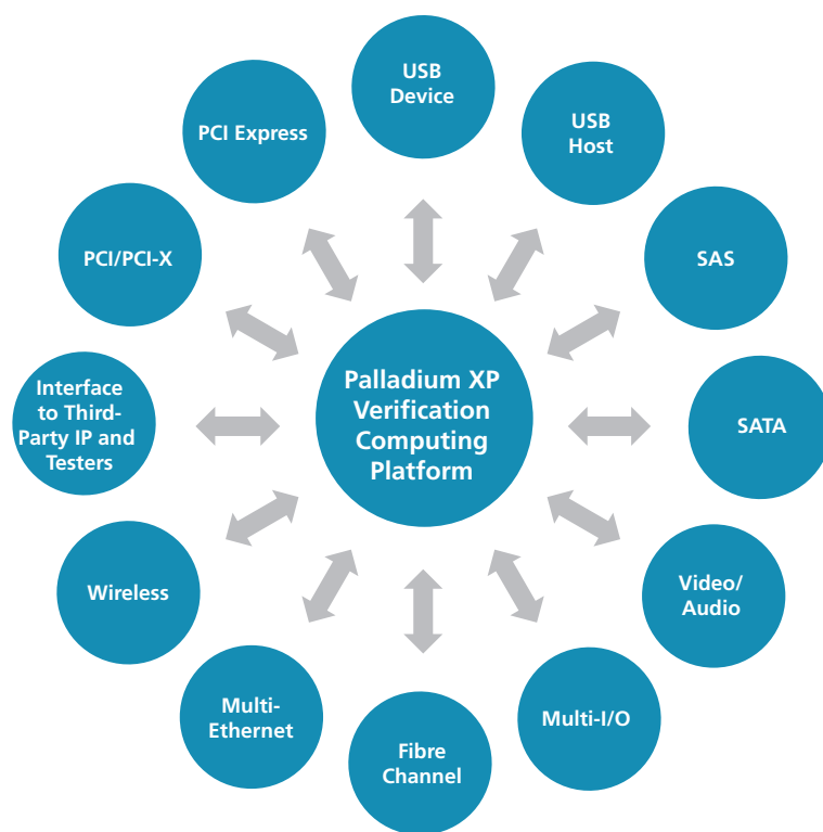
Figure 8: For most industry-standard protocols, off-the-shelf VIP such as SpeedBridge Adapters are available, enabling SoC designs running on Palladium XP to interface with real-world devices/targets/testers for system-level verification
